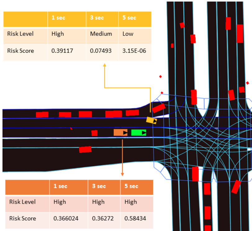
Figure 5.1: An instance of the Lyft Level5 dataset (Houston et al., 2020). The green rectangle represents the ego vehicle, the yellow rectangle is the agent whose risk value is predicted relative to the ego vehicle. The orange rectangle represents another different agent behind the ego vehicle. The tables show the ground truth risk prediction values for 1 second, 3 seconds, and 5 seconds. The black triangle points in the direction the vehicle is moving. In Section 5.2.2, we provide explanations for the risk predicted for the yellow agent.
