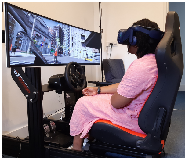
Figure 6.1: Driving simulation setup for the study. Setup included a: VR headset, steering wheel, brake and acceleration pedals, screen, and arcade seat.
