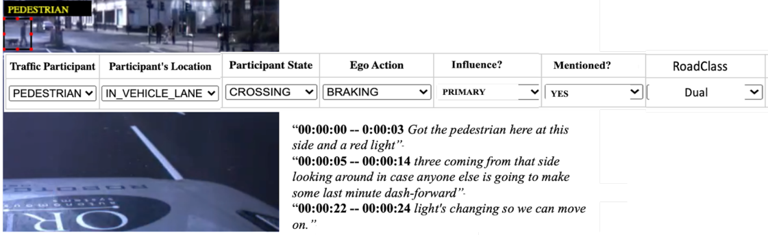
Figure 4.5: An example dataset annotation schema for explanations support. This example assumes that there is a human driver controlling the ego vehicle. The activities of the driver were also noted, e.g., commenting on a scene. The influence tag and the mention tags are introduced. The influence tag indicates whether the agent in question is the primary influence on the AV’s action. The mention tag is used to indicate that the agent was mentioned in the driver’s comment.
